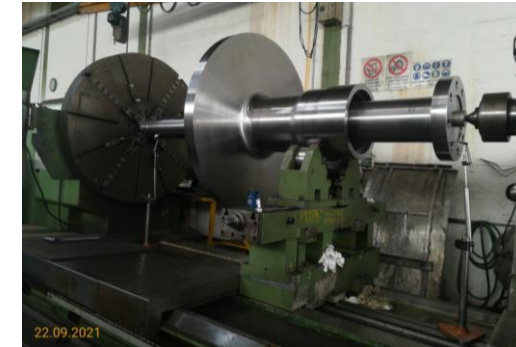
New Waipori 4 rotor shaft being manufactured
